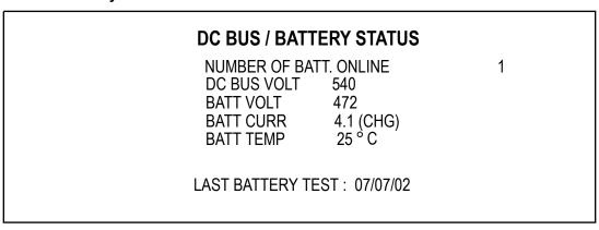
The DC BUS/BATTERY status screen displays the following real-time data:
